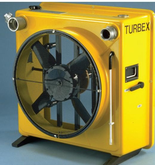
Angus **HI-COMBAT** Turbex MkII High Expansion Foam generators are designed to produce large capacities of high expansion foam, up to 200 cubic metres (7,000 cu.ft) per minute for fast and effective flooding of large and inaccessible spaces with minimal water consumption and subsequently minimal water damage.
