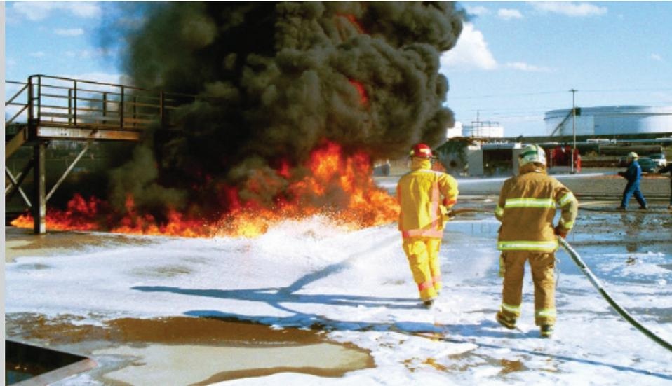
Alcoseal 3-6 is a superior quality Alcohol Resistant Film-Forming FluoroProtein (AR-FFFP) fire fighting foam concentrate for extinguishing and securing flammable hydrocarbon and polar solvent liquid fires.
