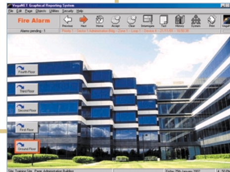
Level 1 page Showing building floor level in alarm
